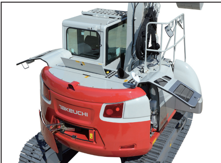
Large Lockable Service Covers Provide Ground Level Access
